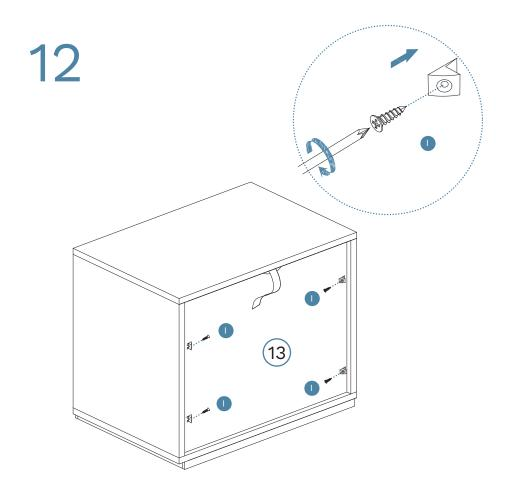
Attach 4 xwedges (I) to panel [13]. Tighten with a screwdriver.
