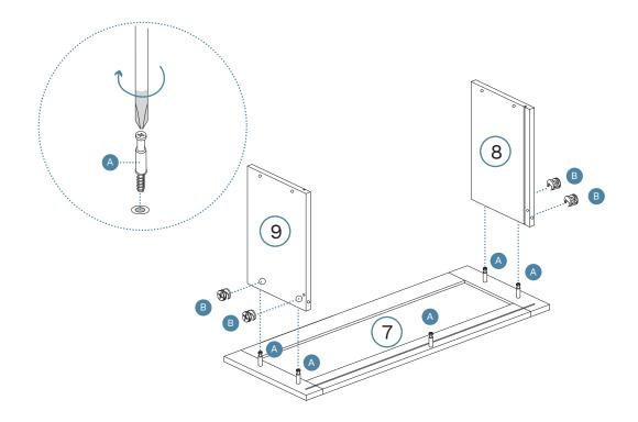
Insert 10 x bolts (A) into panel [7]. Attach panels [8], [9] and [11] to panels [7] and secure with 8 x locking nuts (B). Tighten with a screwdriver.
