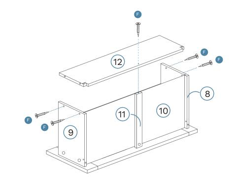
Attach panels [12] to panels [8], [9] and [11] secure with 10 x medium screws (F). Tighten with a screwdriver.
