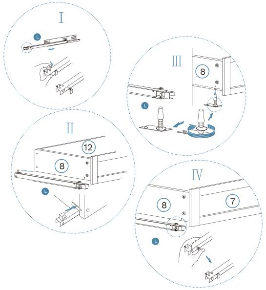
Now both drawers are made up, slide them into rails in the bedside table. Tighten with a screwdriver.
