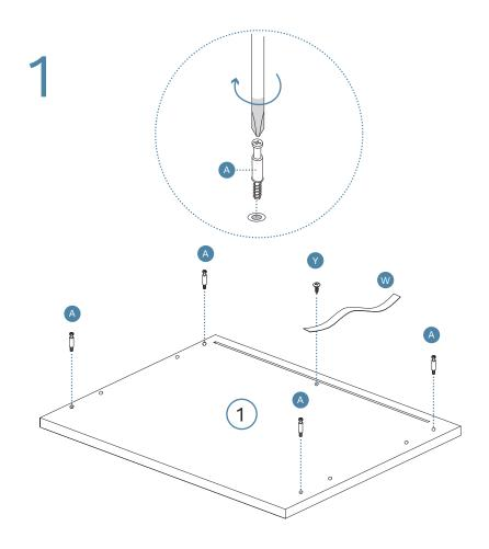
Insert 4 x bolts (A) into panel [1]. Attach 1 x wall strap (W) to panel [1] using 1 x using 1 x screw (Y). Tighten with a srewdriver.
