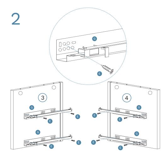
Attach 2 x left slide rails (G) to panel [3] and secure with 4 x small screws (E). Attach 2 x right slide rails (G) to panel [4] and secure with 4 x small screws (E). Tighten with a screwdriver.
